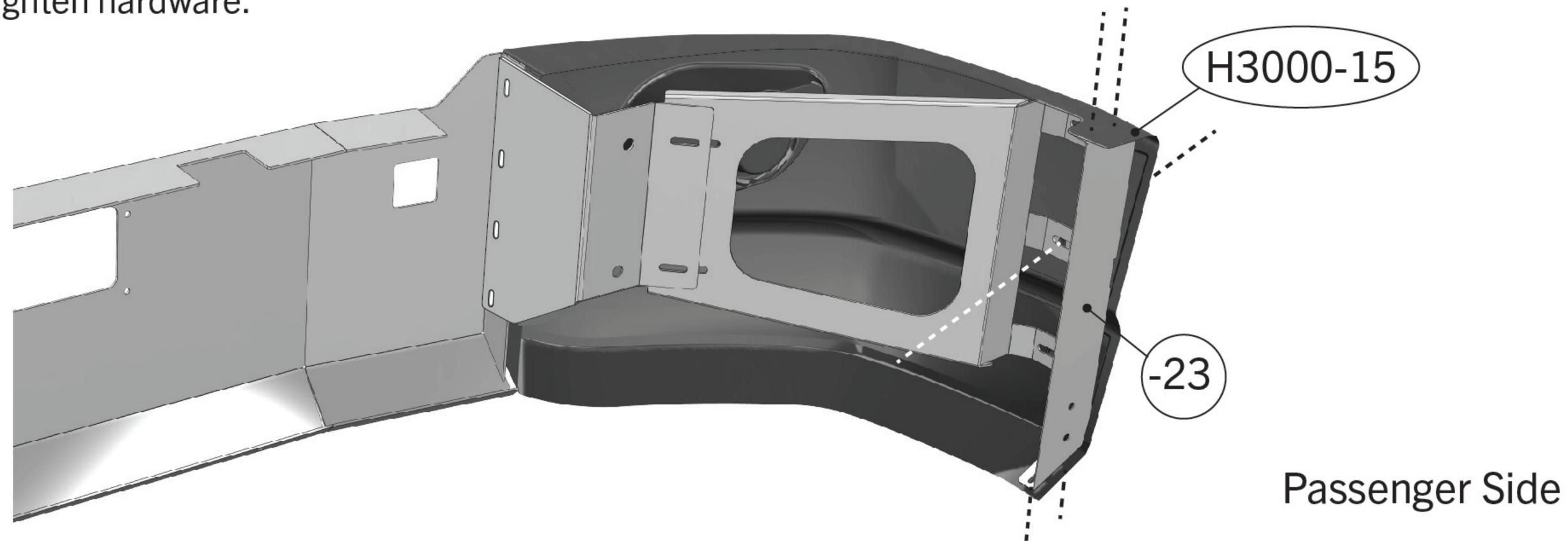
Using HW **08323-125**, **08323-FLAT**, **08323-LOC**, **08323-NUT**, attach lower mounting brackets (**-19**, **-20**) to the (**-23**, **-24**) and to the center section (**H4000-x-02**) on both the passenger and drivers side, ensuring the outer bends face away from the truck. Tighten all remaining hardware.
