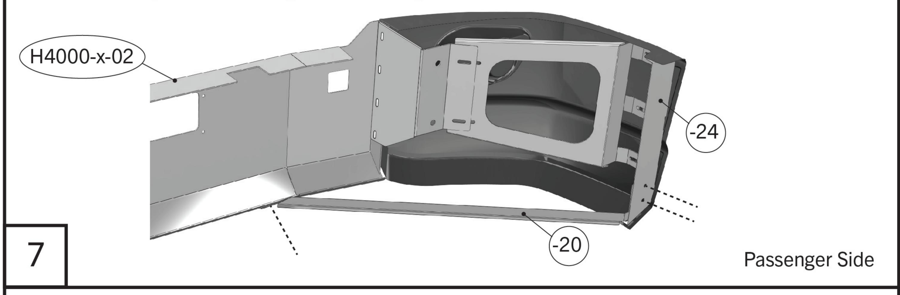
Using HW **08315-FLAT**, **08315-LOC**, **08315-NUT** and (**-21**, **-22**) fog light trim with threaded studs, attach trim through the exterior fiberglass bumper ends (**H3000-15**, **H3000-13**) to the outer tabs of brackets (**-25 & -26 A,B,C**) and (**FOG 1**, **FOG 2**) on the interior of the bumper ends for the fog light assembly as shown.
